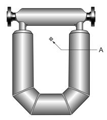
A. Typical center of gravity
