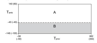
$T_{amb}$  = Ambient temperature °F (°C)  $T_{proc}$  = Process temperature °F (°C) A = All available electronic options B = Remote mount electronics only
