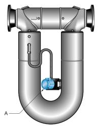
A. Detach electronics from sensor case and mount to a wall or instrument pole
